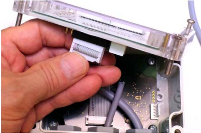
Tighten the cover screws evenly, ensuring that the lid is sealed in position.
