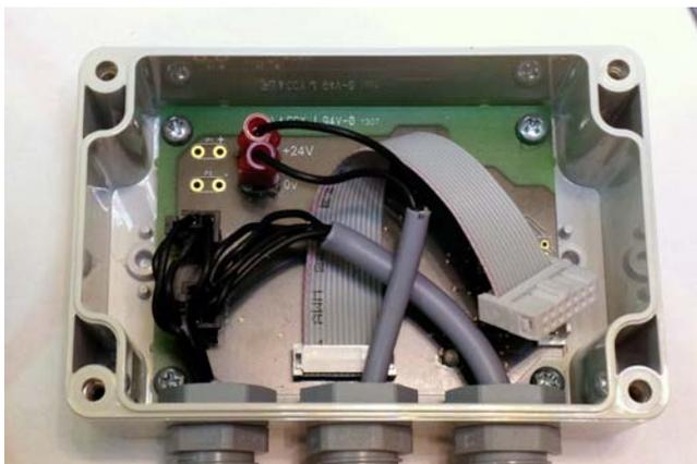
Now, taking the lid, reconnect the ribbon cable connector, and making sure that the white seal is correctly seated in the lid groove, carefully replace the lid.
