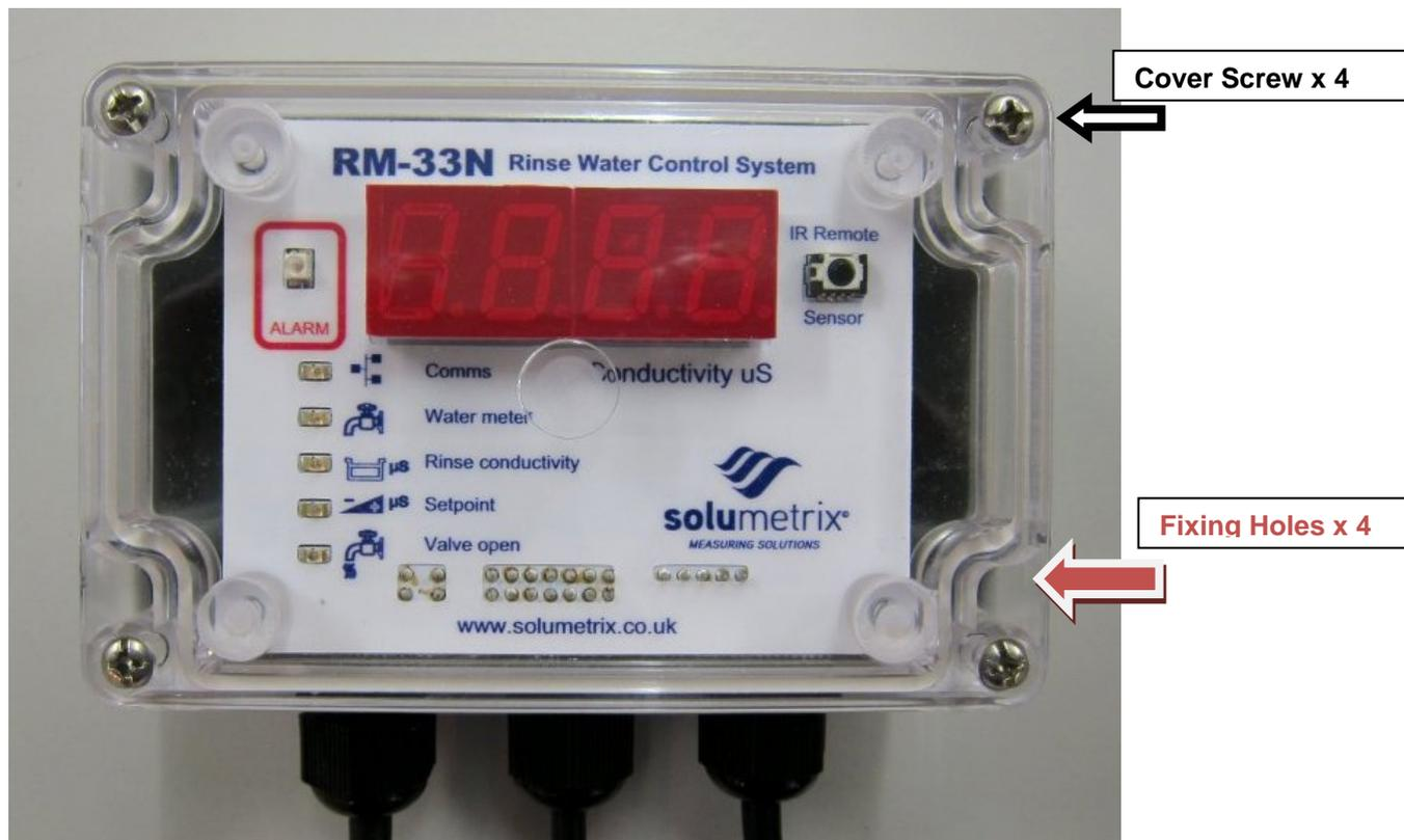
**Fig.3a – the control unit**
