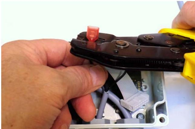
Push the connectors firmly onto the male terminals on the pcb, taking care to put the +24VDC and 0V on to the correct connectors, as shown on the PCB:-
