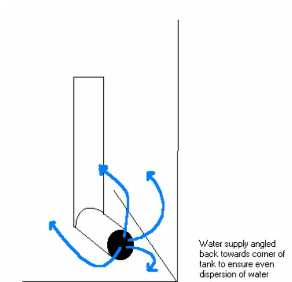
Fig 4.1b – directing water feed pipe.
